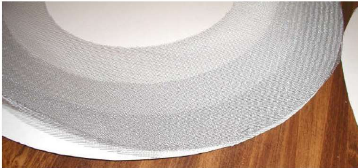
This is a 20-in two dimensional apodizer made of window screen
