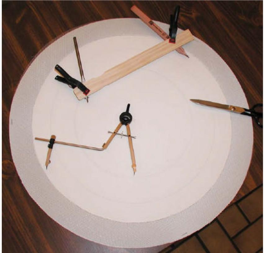
*For big instruments you sometimes need to construct your own compass, as was done here using a paint stirrer, a carpenter's pencil, a wood drill, and clamps.*
