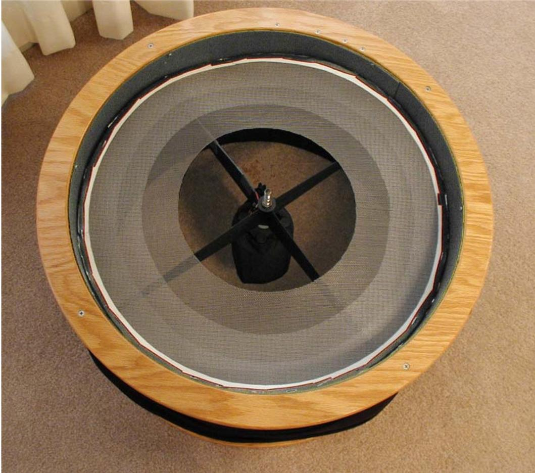
*The picture shows how the screen is used at the upper end of the telescope. I like these "minimalist" screens because they don't involve enough hardware to seriously unbalance the telescope.*
