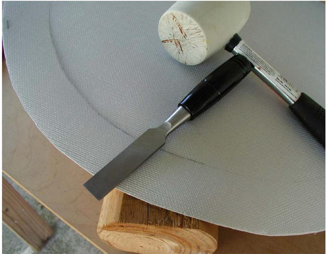
After each of the annuli are cut out, separate them by removing staples from their cut backings. Attach them to the fourth backing with all radii drawn-in from the outside in. Here, I put the 8.5-inch inside radius first, followed by the 7.05 inch radius. The
