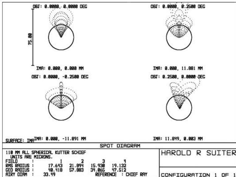
Figure 3: Spot diagram of 2-mirror, 110-mm Kutter schief
