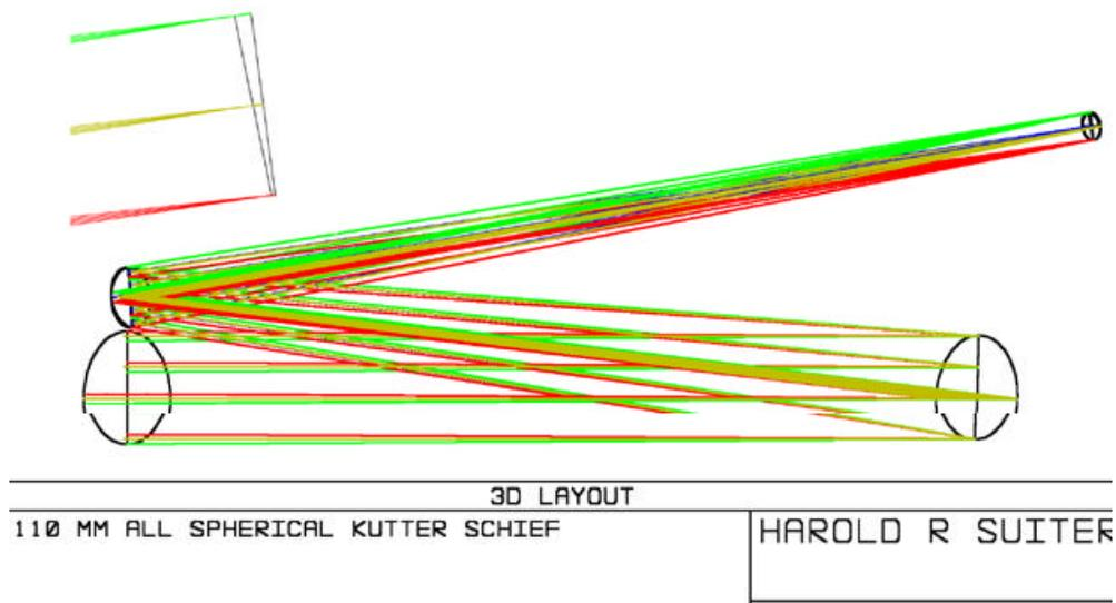
Figure 2: The 2-mirror, 110-mm Kutter schiefspiegler anastigmat
