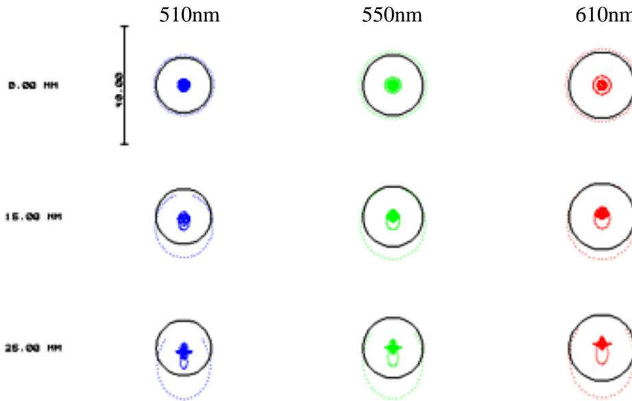
Figure 6. Spot diagram of big separated secondary Mak-Cass.
