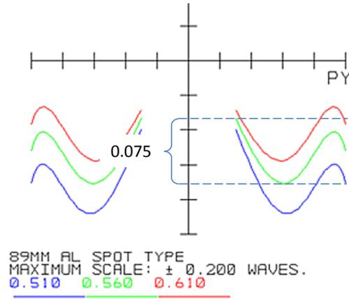
Figure 3. Residual on-axis optical path difference of 89-mm f/16 depicted in Figure 2. Strehl ratio of this objective is 0.98. Full scale = 0.2 wavelengths.
