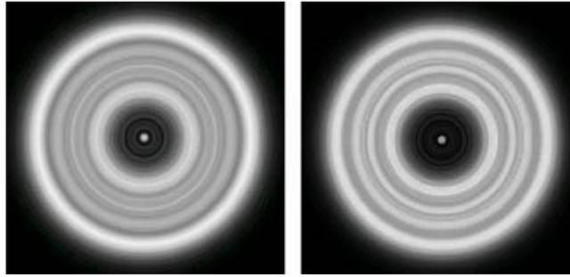
Figure 4. Calculated star test of a good Maksutov telescope, showing subtle difference that would likely go unnoticed when viewed serially.
